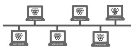
other. For a major disruption to take place, the bus (hub/switch) or a broken cable can result in failure of data-packet transmission to stations. Bus networks are easy to expand and faults are easily detected. That said, a bus
