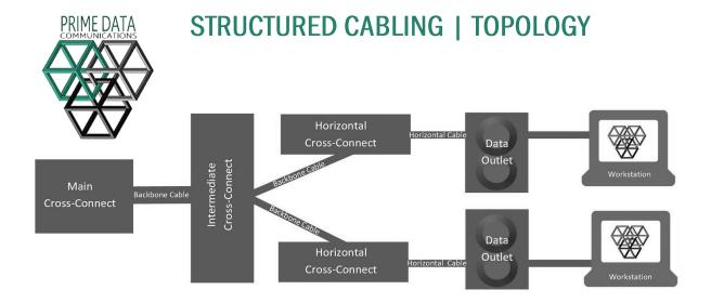
**Horizontal Cabling** runs both horizontally and vertically, conveying voice and data between a source and the end-user. Cable lengths between cross-connects are determined by the type of cable utilized, physical obstacles, data source and type and Prime Data Communications' commitment to uninterrupted connectivity.
