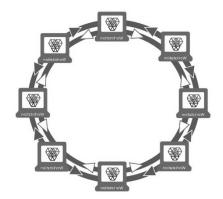
**Ring Topology** | computers are basically connected to one another in a circle (with each device having only two neighbors, with data running in one direction or bidirectionally/dual-ring Topology). Ring Topologies can sustain large networks much more effectively than a bus. And, when bidirectional, can provide an extra layer of protection against failure; with dual-rings providing packet-backup if the first ring goes down.
