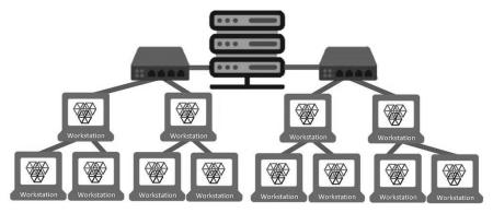
Tree Topology | yes, this is network with roots and branches - the parent-child schema is favored for Wide Area Networks to sustain lots of spread-out devices. Tree topologies can be used to extend both Bus and Star Topologies. The format makes troubleshooting more succinct because performance issues can be spotted by systematically
